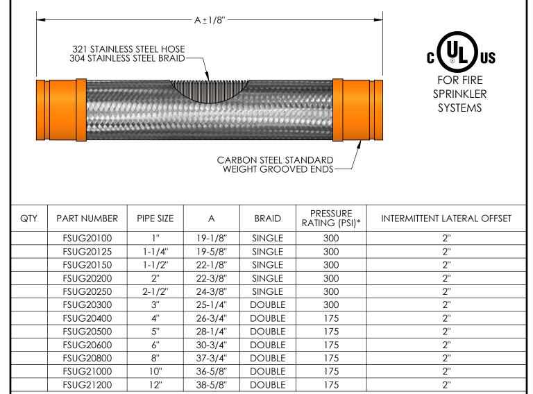
SUITABLE FOR USE IN DRY PIPE SYSTEMS TEMPERATURES TO -40°F
